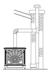
Figure 23 - Vertical Venting Configuration Through Chimney
